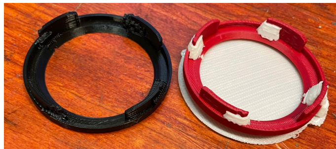
Figure 5: Retaining ring for trackball from a console input device in the operational section of the ship.
